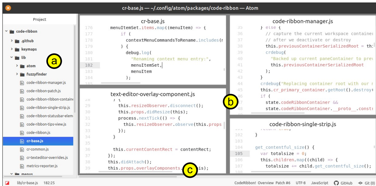
Fig. 1. The CodeRibbon interface as an Atom plugin composed of (a) Atom’s standard file listing, (b) CodeRibbon’s grid of code documents showing a resized 2x2 configuration, and (c) there are many more documents to the right that are off screen, that can be navigated to using keyboard shortcuts or a horizontal scrollbar. Navigating to these off-screen documents works like an animated carousel.
